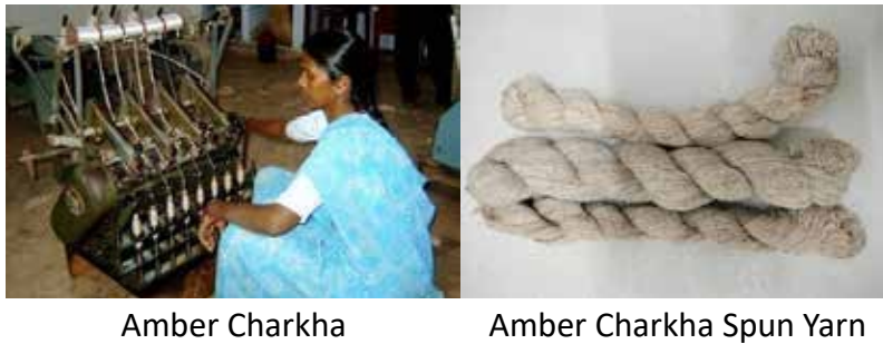
Figure 5: Spun yarn preparation through Amber Charkha
