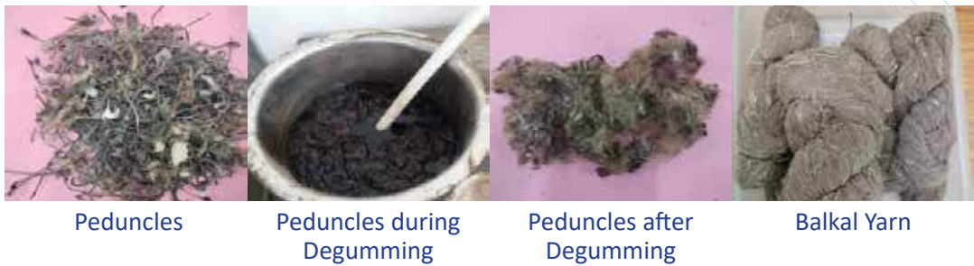
Figure 6: Steps involved in processing of peduncles
