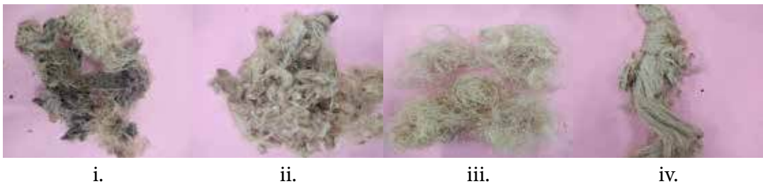
Figure 4: -Various types of reeling & post-reeling waste; i) deflossing waste ii) reeling waste iii) re-reeling/winding/weaving waste & iv) Warping/drawing waste
